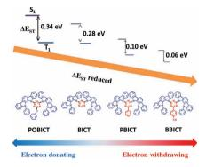
A series of indolocarbazole/1, 3, 5-triazine hybrids are designed and prepared as hosts for phosphorescent orangeemitting diodes. Singlet-triplet splitting and carrier injection/transporting are adjusted by introducing moieties with different electronegativity. By harmonizing the optical and electrical properties, high efficiency with ultra-low roll-off is realized in the device.
