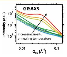
The relationship between donor crystallization and blend phase separation is investigated in solution-processed bulk heterojunction organic solar cells using in-situ thermal annealing grazing incidence X-ray scattering. Based on these data as well as blend electrical properties measured as a function of annealing temperature, it is hypothesized that donor crystallization is the driving force for the development of blend phase separation.
