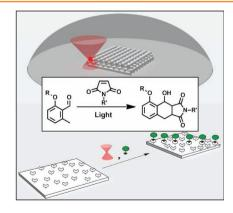
A light-induced Diels-Alder reaction is employed for the fabrication and the spatially resolved surface patterning of 3D microstructures using a direct laser writing setup. Woodpile photonic crystals with a lateral rod spacing of 700-500 nm are fabricated and characterized via SEM, FIB milling, and transmission/reflection spectroscopy. Covalent surface patterning of the KIT-logo is verified using ToF-SIMS.
