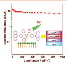
Grafting dimesitylboryl groups onto 2,3,4,5-tetraphenylsiloles generates efficient bifunctional materials that can simultaneously serve as light emitters and electron transporters in OLEDs. Remarkably high electroluminescence efficiencies up to 13.9 cd  $A^{-1}$ , 4.35% and 11.6 lm  $W^{-1}$ are attained from the double-layer OLEDs based on them.
