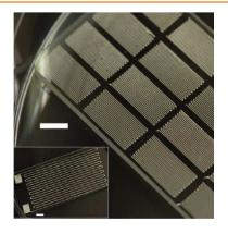
A novel method for directly writing liquid gallium-indium alloy is presented. In addition to the basic characterization of the direct writing process, a design algorithm for process stability is also developed. The method is employed to fabricate a strain gauge exhibiting an approximately linear behavior through strains of 50% with a gauge factor of 1.5.
