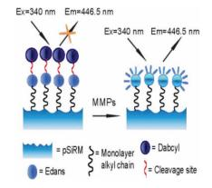
An optical biosensor based on functionalized porous silicon resonance microcavity (pSiRM) using matrix metalloproteinase (MMP) substrate containing a fluorophor and a quencher is demonstrated. The presence of MMP cleaves the substrate leaving the fluorophor on the pSiRM matrix which is now emitting the fluorescence. This biosensor sensitively and selectively detects the MMP in buffer solution and human wound fluid.
