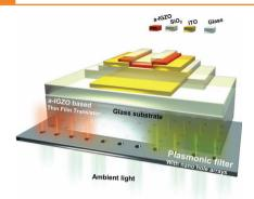
amorphous-indium-galliumnovel zinc-oxide-based application with stable switching characteristics under negative bias illumination is shown. Metallic nanohole-based plasmonic filters are used for tuning the spectrum of the ambient light source, and the photosensitivity of the a-IGZO-TFT is investigated within a selectively controlled spectral range. The suggested thin-film transistors show greatly improved stability even in a negative bias illumination stress environment.
